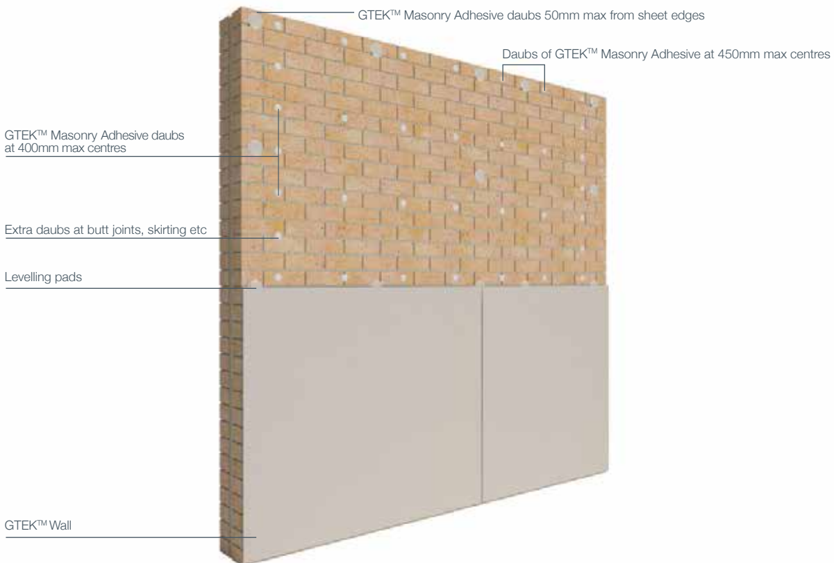
FIGURE 4 – ADHESIVE APPLICATION HORIZONTAL SHEET FIXING
