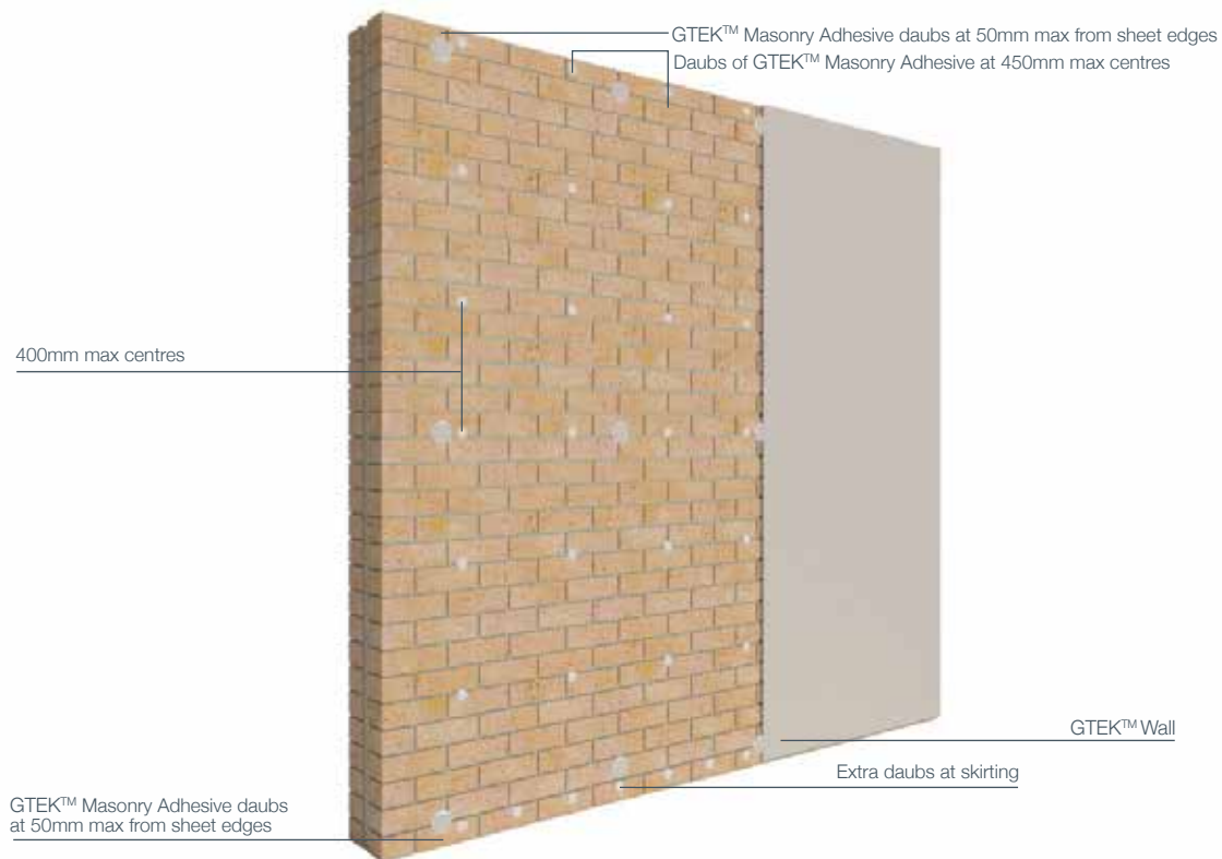
FIGURE 6 – ADHESIVE APPLICATION VERTICAL SHEET FIXING
